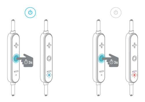
To power on your BE Sport3, press Power/Function button for about 3 seconds until the LED indicator flashes blue and you hear the "Power on" when voice prompt is activated or a beep if the voice prompt is not used. *NOTE:*
